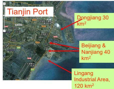
More than **190 km<sup>2</sup>** of land has been reclaimed for the **Tianjin Port** in Tanggu using clay slurry
